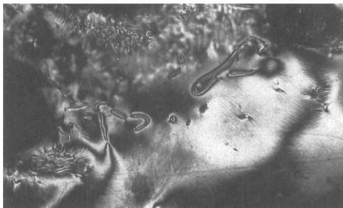
FIGURE 2 Polarized light micrograph of 3 at 200°C, nematic schlieren texture, 160 \times .
